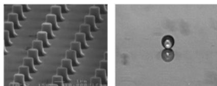
Figure 12. Substrate decorated with posts (the bar indicates 1  $\mu$ m). If coated with a monolayer of fluorinated silanes, this substrate is found to be super-hydrophobic [37].
