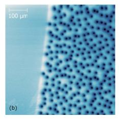
Figure 1 | Images of vortices in 200 nm thick YBCO film taken by Scanning SQUID Microscopy after field cooling at 6.93  $\mu$ T to 4 K. (b) is taken after heating above  $T_c$  and re-cooling. The sample edge at the left side of the images is used as a reference for scan location.
