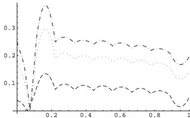
Figure 4: Error  $|p - p_9|$  with our method for Example 2: (---)  $d = 0.01$ , ( $\cdots$ )  $d = 0.025$ , (- $\cdot$ -)  $d = 0.033$ .
