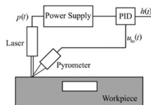
FIGURE 1. Pyrometer process control of laser surface hardening
