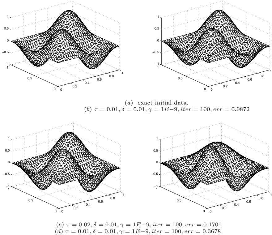
FIGURE 7. 2D reconstruction in example 4. (a) exact initial data, (b) and (c) comparison with different starting time,  $\tau=0.01$  and  $0.02$  respectively, with measurement in  $\omega = (1/4, 3/4) \times (1/4, 3/4)$ , (c) and (d) comparison with different positions of the observation regions,  $\omega = (1/4, 3/4) \times (1/4, 3/4)$  and  $\omega = (1/8, 5/8) \times (1/8, 5/8)$  respectively, with the starting time  $\tau=0.01$ .
